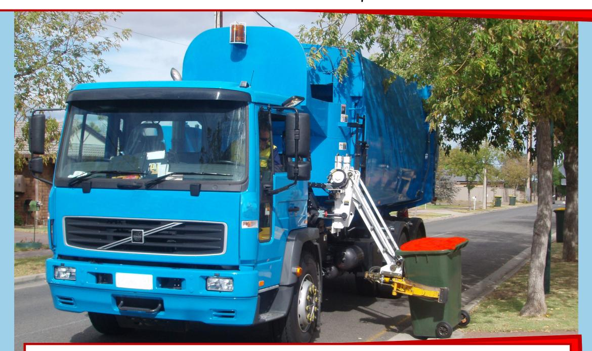
A truck picks up the bin and tips the waste into the truck.
